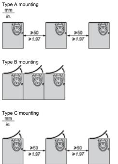
By removing the protective blanking cover from the top of the drive, the degree of protection for the drive becomes IP21. The protective blanking cover may vary according to the drive model, see opposite.
